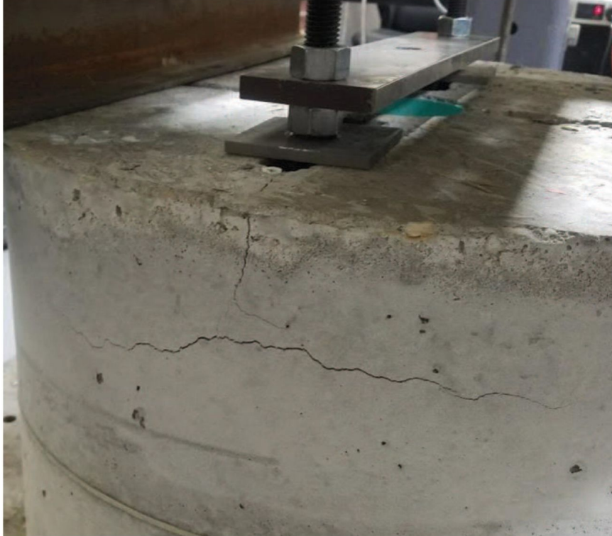
Figure 4: Typical Cracking Pattern
